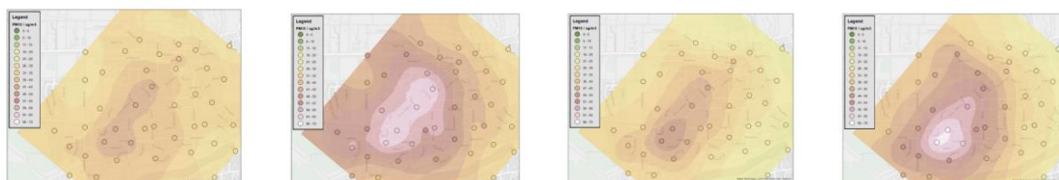
Figure 4-1: 24-hour mean PM 2.5 concentrations from 40 monitors (including interpolated contours) for four example consecutive days in June 2023.
