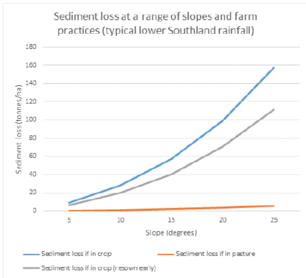
Figure 1, erosion of a typical Southland farm by slope
