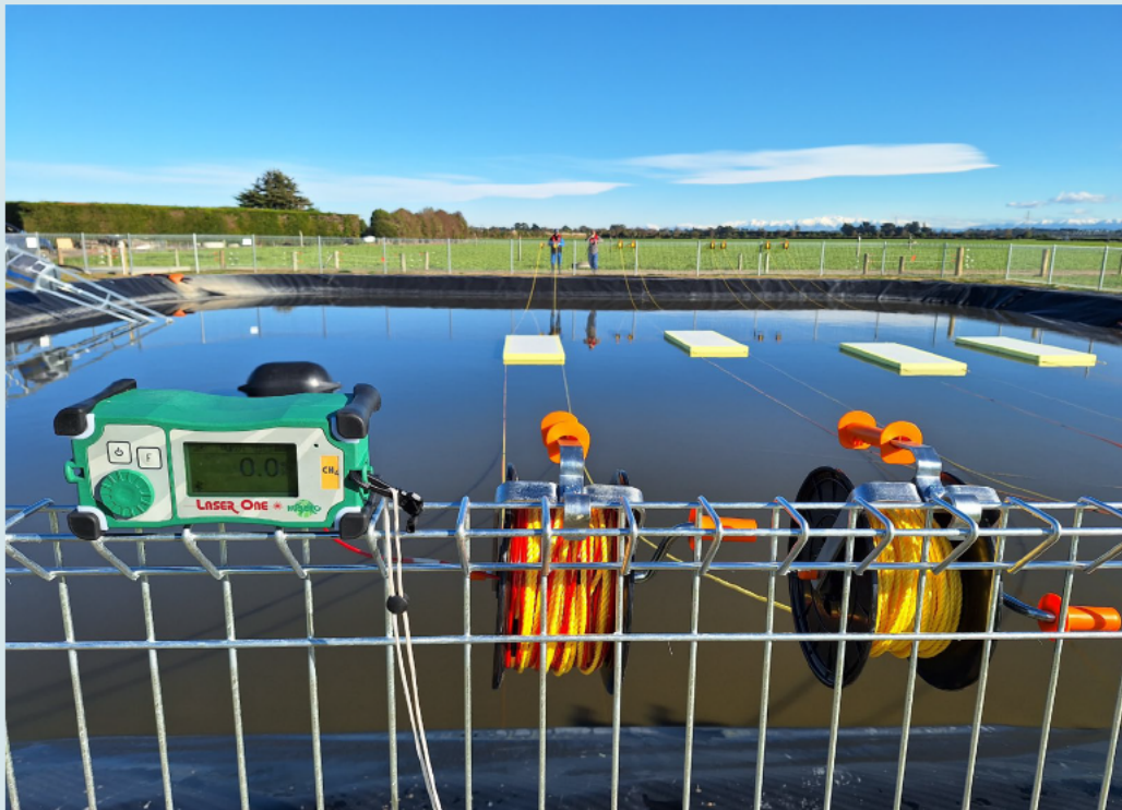
Image: Measuring methane emissions on an effluent pond
