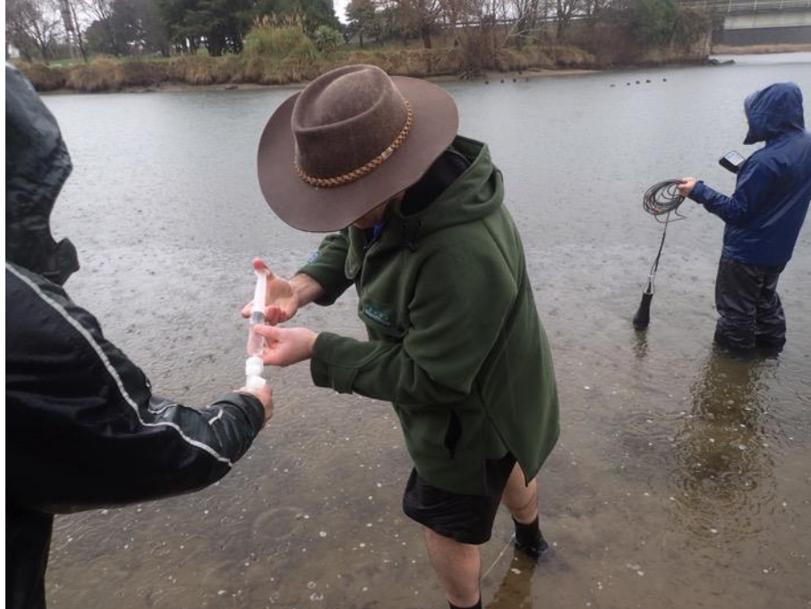
Figure 4: Taking water samples for nutrient analysis (foreground) and using a multiparameter probe to measure the physical and chemical parameters (background) within the Waikouaiti River.
