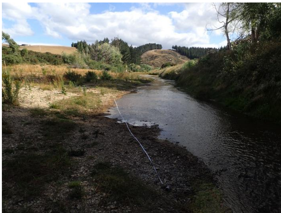
Figure 2: Ten metre transect line along the Waikouaiti River indicating the sampling area for site characteristics and the wider ecological survey.
