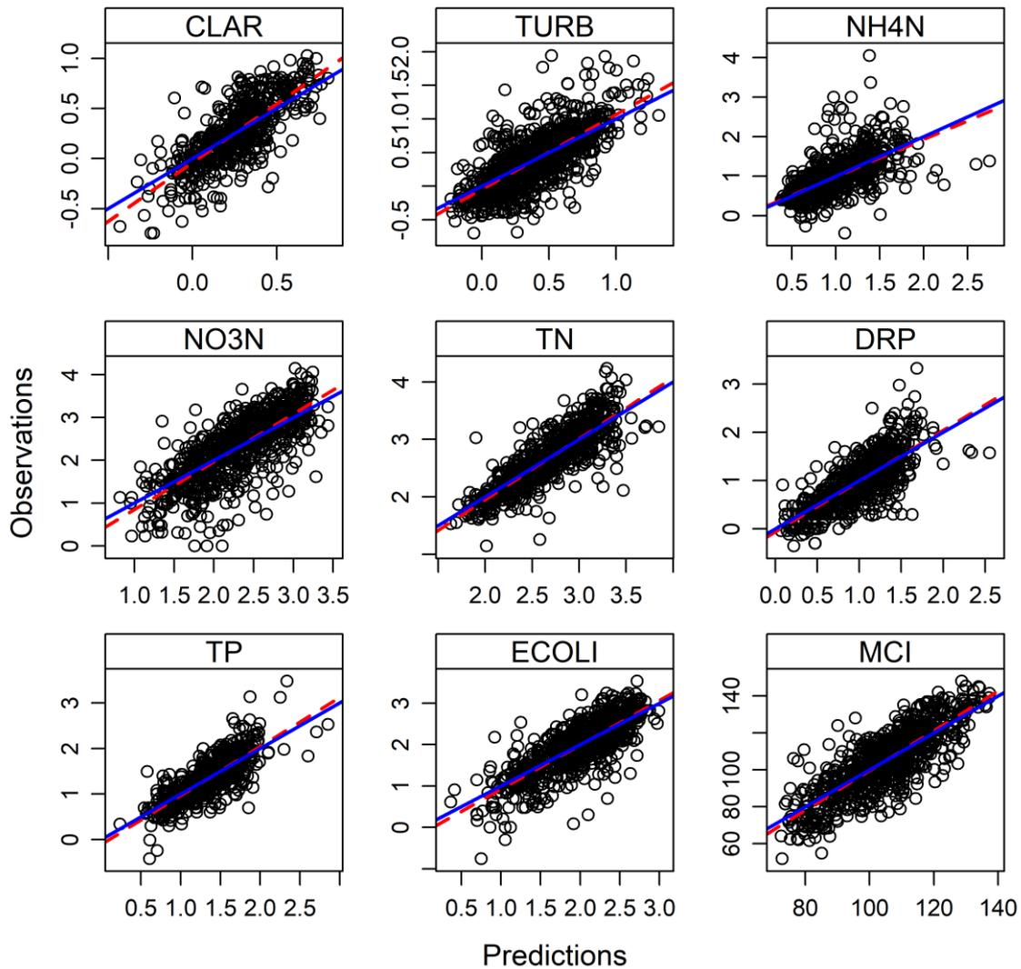
**Figure 4-1: Comparison of observed water quality versus values predicted by the random forest models.** Note that the observed values are plotted on the Y-axis and predicted values on the X-axis, following Piñeiro et al. (2008). Red dashed line: best fit linear regression of the observed and predicted values. Blue solid line: one-to-one line. Units are the  $\log_{10}$  transformed units of all water quality variables except for MCI, which uses non-transformed values.
