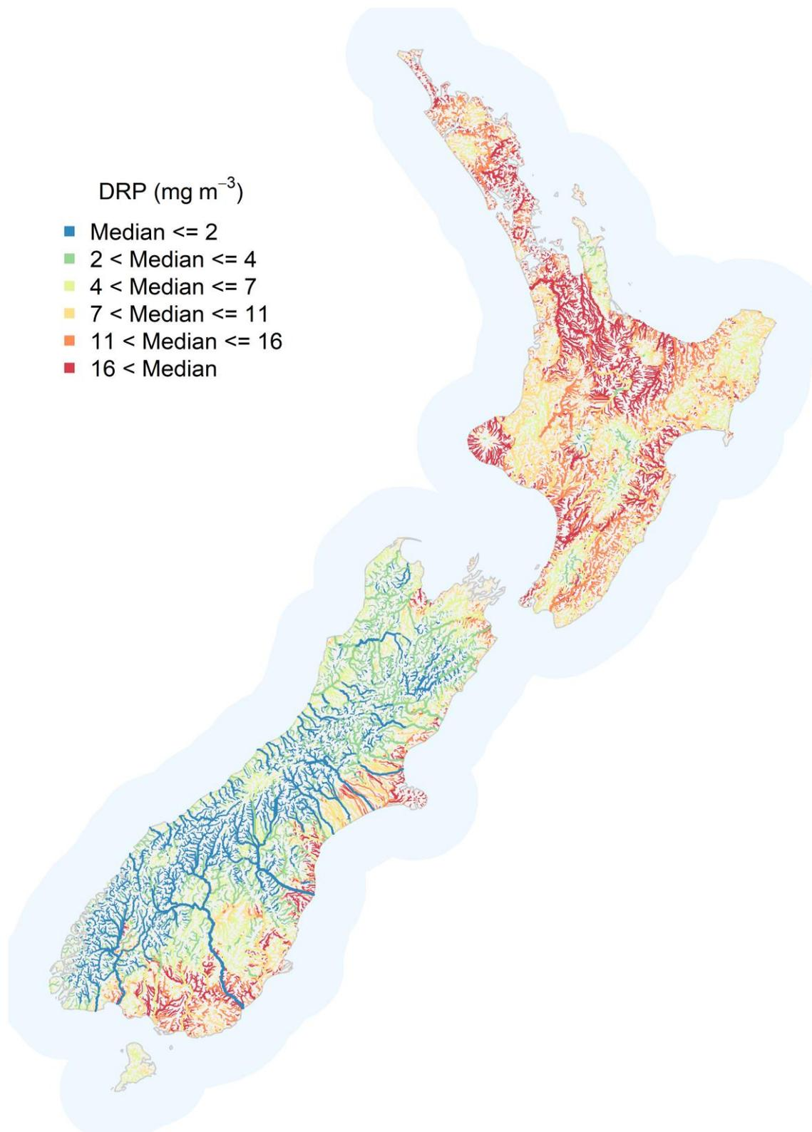
**Figure 4-11: Predicted median DRP concentration in New Zealand rivers.** Map shows all nzsegments of Order 3 and higher. Smaller rivers are omitted to make river networks distinguishable.
