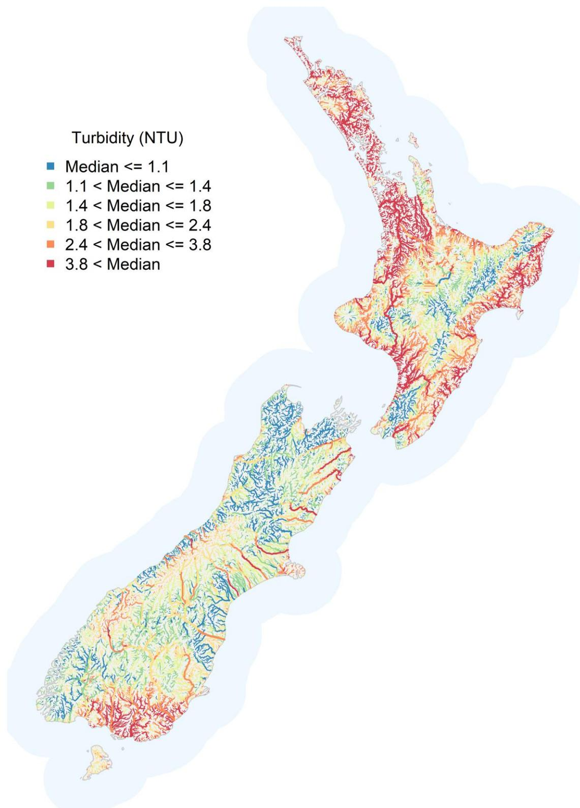
**Figure 4-7: Predicted median TURB in New Zealand rivers.** Map shows all nzsegments of Order 3 and higher. Smaller rivers are omitted to make river networks distinguishable.
