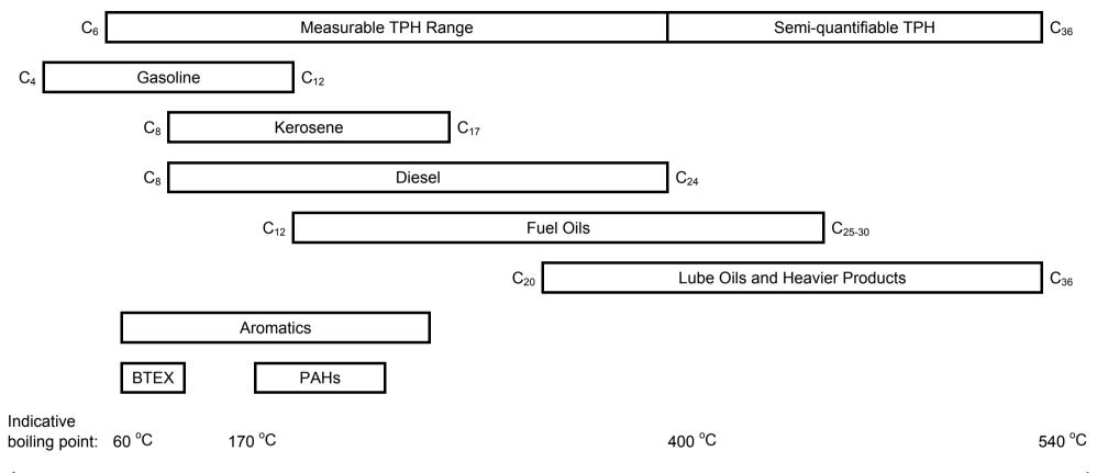
This diagram shows the typical carbon number ranges of common products, together with indicative boiling points. This is contrasted against the detectable range of a TPH analysis.
