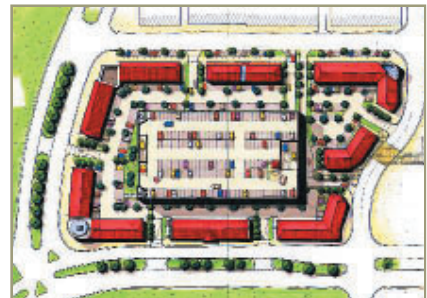
Here at Manukau, a multi-storey car park will have offices and apartments screening it from the street.
