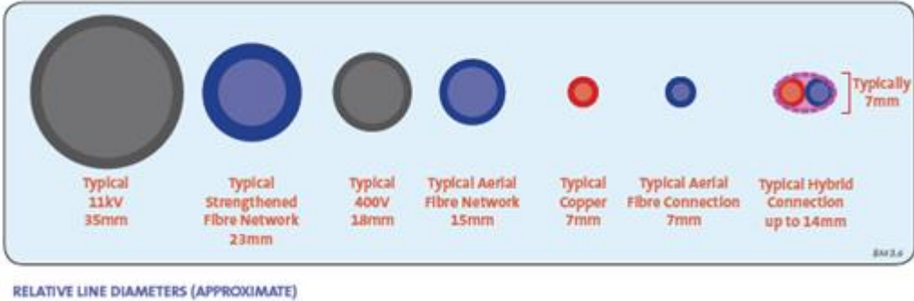
Figure A2.3: Diagram comparing cable sizes (not to scale)
