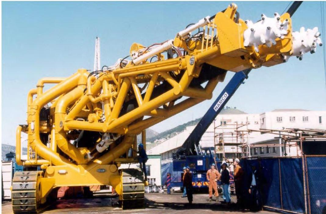
**Figure 3-3: Example of sub-sea extraction crawler demonstrating scale.** From TTR Supporting Information for Marine Consent Application<sup>2</sup>.
