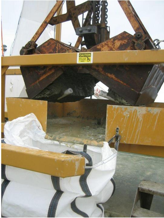
**Figure 3-2: Bulk sampling of phosphorite nodule bearing sediments on the Chatham Rise.** Image courtesy of CRP.
