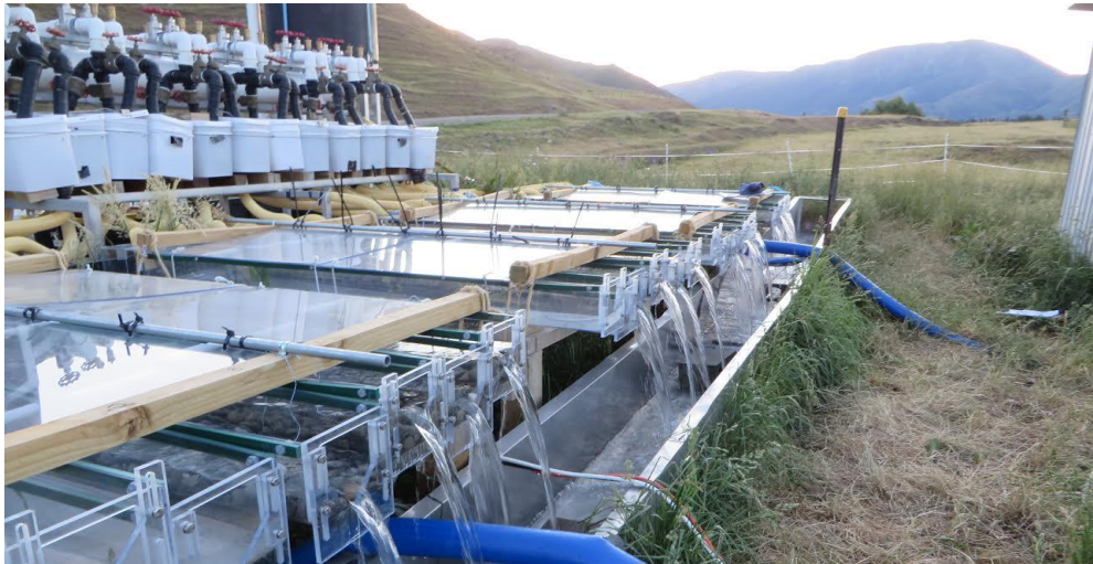
Figure 28. The NIWA flow through channels.
