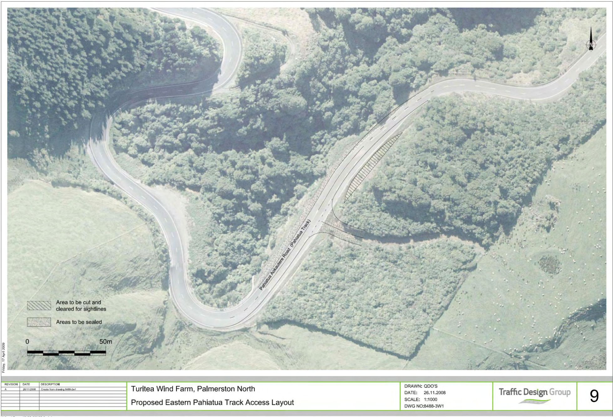
Appendix 5: Pahiatua-Aokautere Road – Eastern Site Access (TDG drawing 8488-3W1, Sheet 9, Revision A)
