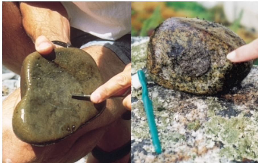
Figure 8: Sampling periphyton from a defined area on the surface of a stone. Left: scraping the diatom film from within circumscribed area to show the difference in colour of the sampled area within the circle and the diatom film (additional scrubbing with a coarse toothbrush will complete the sampling). Right: a defined circle of periphyton mat which will be scraped/brushed off into a container as the sample.
