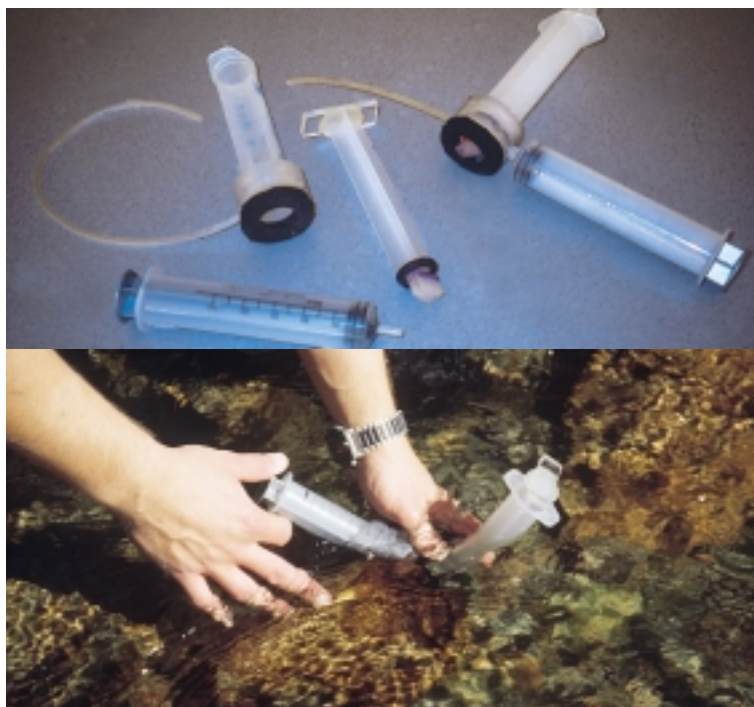
Figure 9: Double syringe periphyton sampler. Top: the apparatus, showing the components, and an assembled set. Bottom: the device in position in a stream ready for use.
